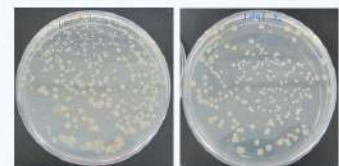
Figure 2: Comparison of diversity in bacterial colonies of samples from mechanical filter at day 1. Right UV ON and Left UV OFF
