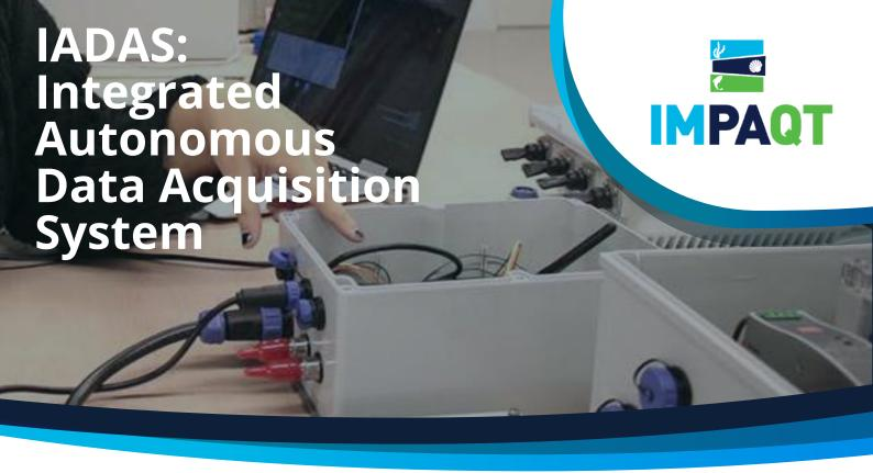
The IADAS is an electronic device designed to collect and transfer data from physical sensors in an autonomous manner to support the digitalization of the aquaculture data decision process.
